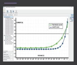
The characteristics of the large-area device can be compared to the local I-V curve
