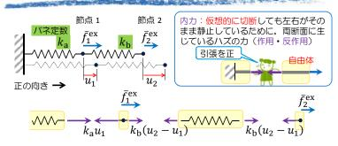
• 節点1の静止条件:  $(-k_a u_1) + k_b (u_2 - u_1) + \bar{f}_1^{\text{ex}} = 0$
