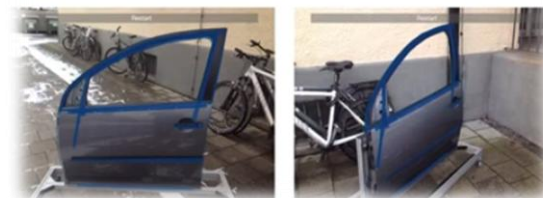
3-D Markerless Tracking based on CAD data
