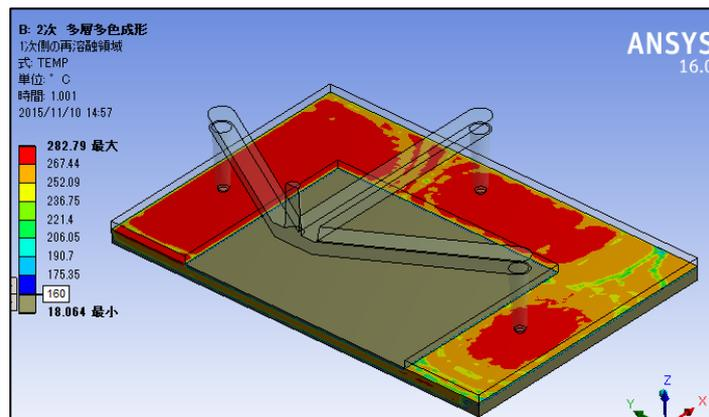
Figure 1: Temperature profile of the re-melted areas (160 °C or more) of the product of the first molding
