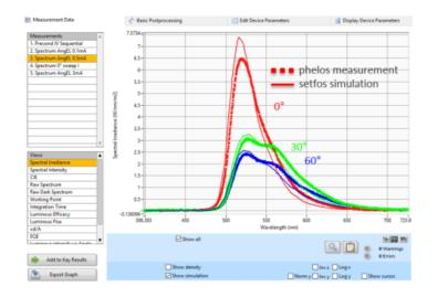
Setfos dipole emission and drift- diffusion model can be run directly from the Phelos control GUI.\*
