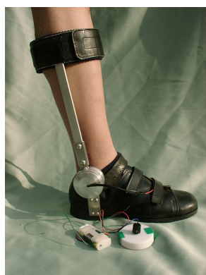
Fig. 7 Controllable AFO with SCMRB-1
